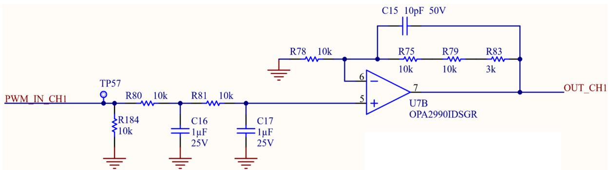
At each input of each channel a PWM from Portenta is provided filtered by a double low pass filter, obtaining a DC output with a small AC ripple. The signal is then fed to the channel non inverting amplifier which amplifies it by 3.3.
